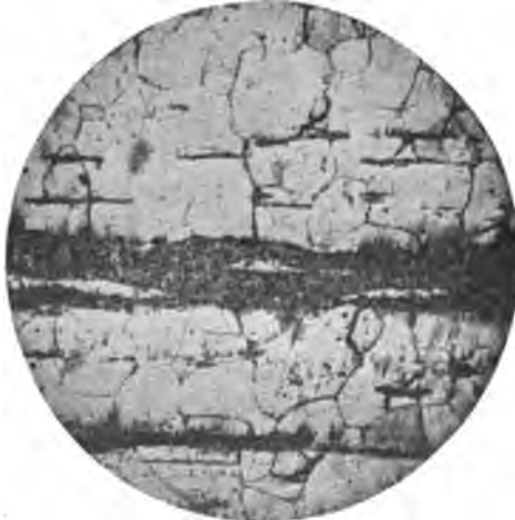
FIG. 13. — Wrought Iron. Longitudinal Section. Magnified 100 Diameters. (Boynton.)
